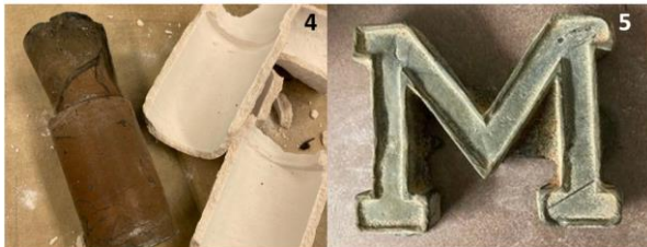
Fig. 4 & 5: (4) Basalt cylinder poured and annealed in a silica-based ceramic mold. (5) Basalt “M” poured into an open-faced green sand mold and annealed.
