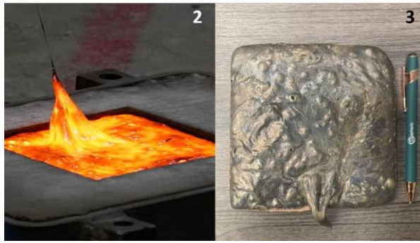
Fig. 2 & 3: (2) Molten regolith poured into a green sand mold and (3) the result of that pour after annealing.
