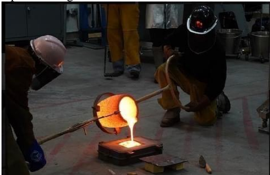
Fig. 1 Basalt pouring into an open-faced green sand mold.
