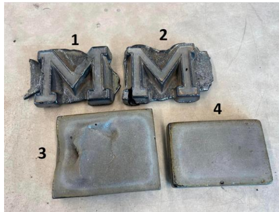
Fig. 6 Basalt/anorthosite mix pour into a green sand mold and annealed. Slight warping from removing the molten material from the mold and placed into the kiln.
